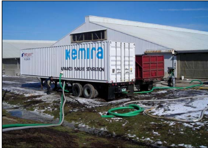
Figure 6. The Kemira manure dewatering system, enclosed in trailer.
