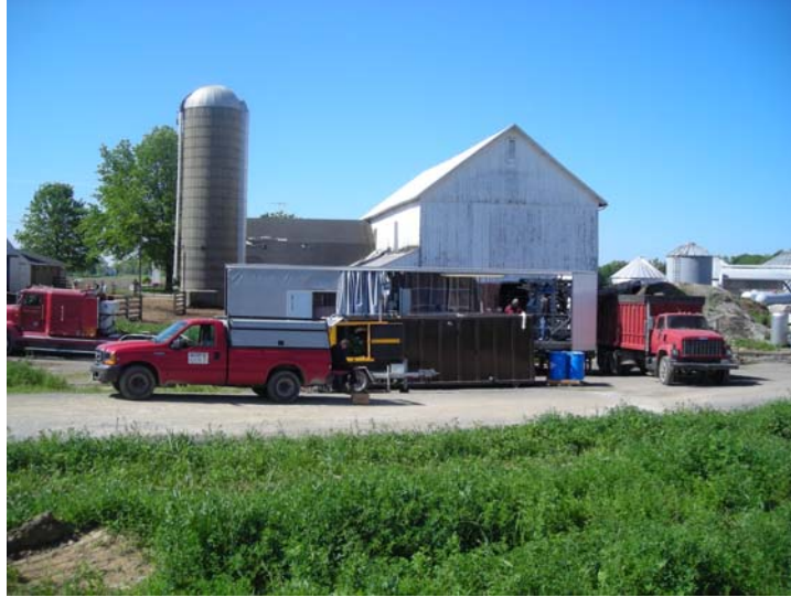
Figure 4. MSD Environmental Services portable Belt Press at Royer Farm
